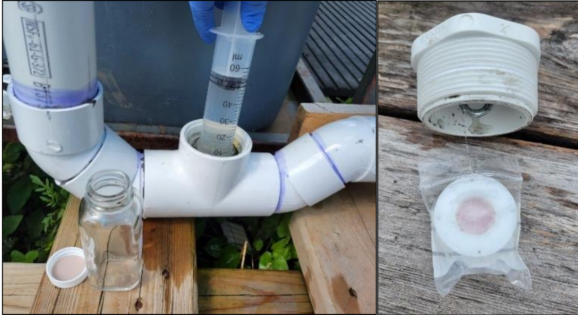
Figure 2.5 Water sample (left) and DGT passive sampler (right) positioned at outflow of artificial stream.
