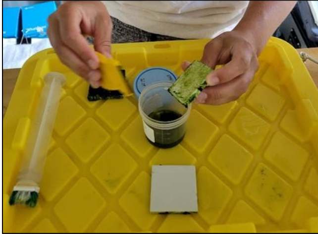
Figure 2.6 Scraping biofilm off ceramic tiles into a specimen cup using a toothbrush and mini glass scraper.
