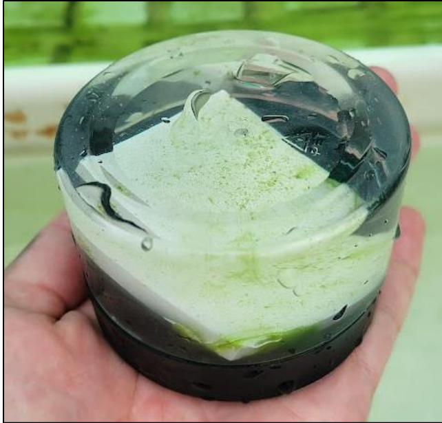
Figure 2.8 An SRP uptake chamber containing one biofilm-colonized tile and stream water.
