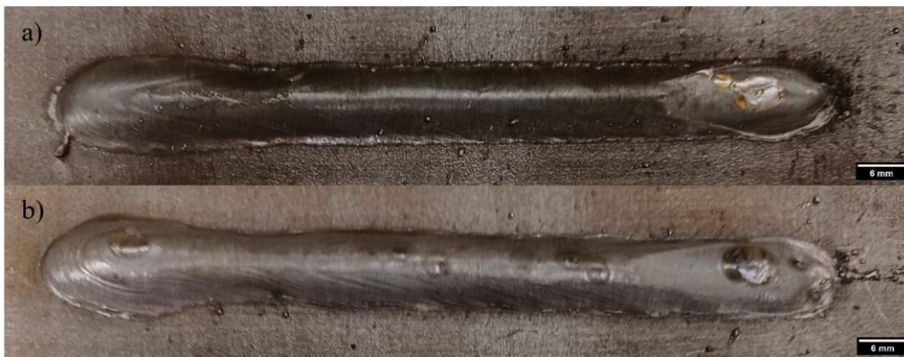
Figure 6-42 a) Aerial view of the weld bead produced during GMAW taken after the experiment to measure its width. b) Aerial view of the weld bead produced during DCW-GMAW taken after the experiment to measure its width.
