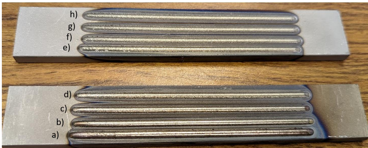
Figure 6-5 Single track LDED experiments to correlate cooling rate to microstructure of 431 stainless steel
