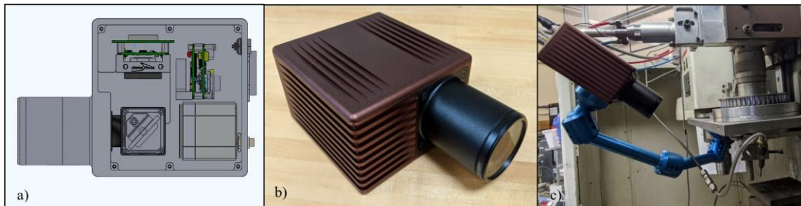
Figure 3-2 a) Final MOC sensor CAD model b) MOC sensor prototype c) Prototype mounted in the ALFa Laboratory
