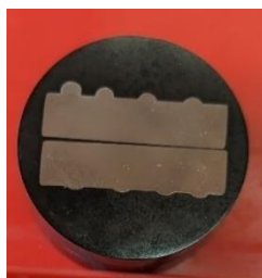
Figure 6-7 Cut and polished specimens with 431 stainless steel depositions
