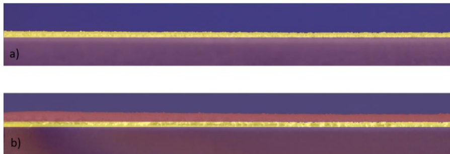
Figure 5-18 Macro imaging and segmentation used to measure the real clad geometry. a) first layer of deposition, with clad highlighted in yellow and substrate in red. b) second layer of deposition with the height of the first layer highlighted in yellow to demonstrate the difference, which is the added material.
