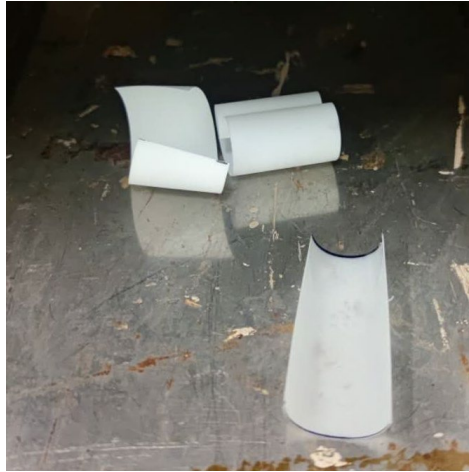
Figure 2-7: The curvature of APF-500 when the curing temperature is 100 °C. The melting points of the adhesive layer and printing layer are around 90 °C and 150 °C, respectively.
