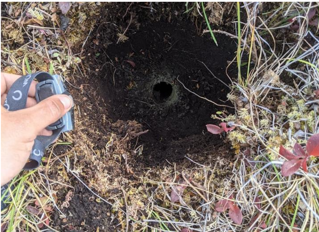
Figure 2.7: A soil transect example: drilled hole shown in the middle that shows a change in colour delineating the peat and mineral soil boundary.
