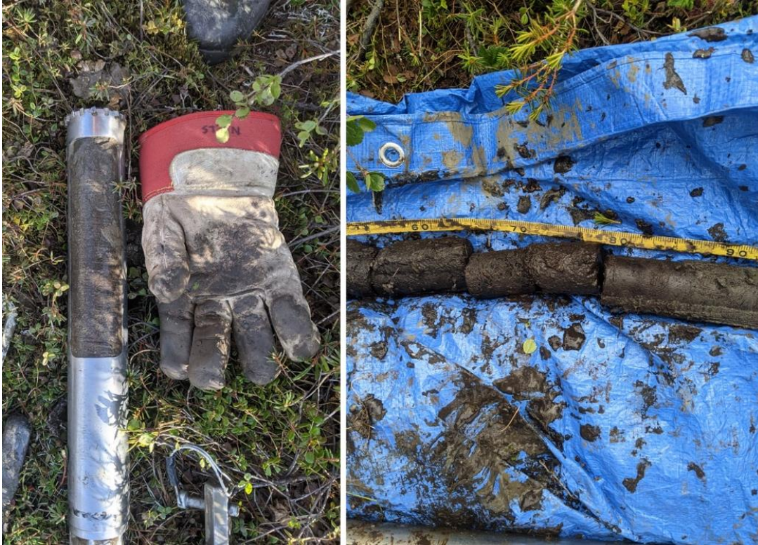
Figure 2.5: A photo of the coring extension used by the drill on the left, as well as how the cores were laid out in the field to be recorded.
