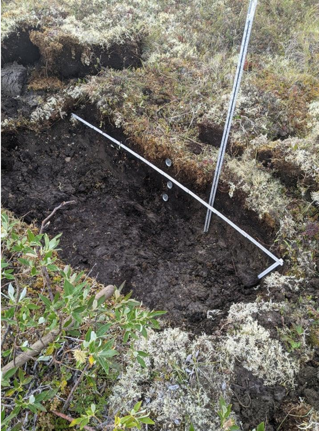
Figure 2.6: A soil pit in the Siksik Creek catchment showing how soil depths and temperature were measured. To note, an inter-hummock zone marked by the redder mosses is surrounded by the lighter lichens, which happened to lay over top of the hummocks.
