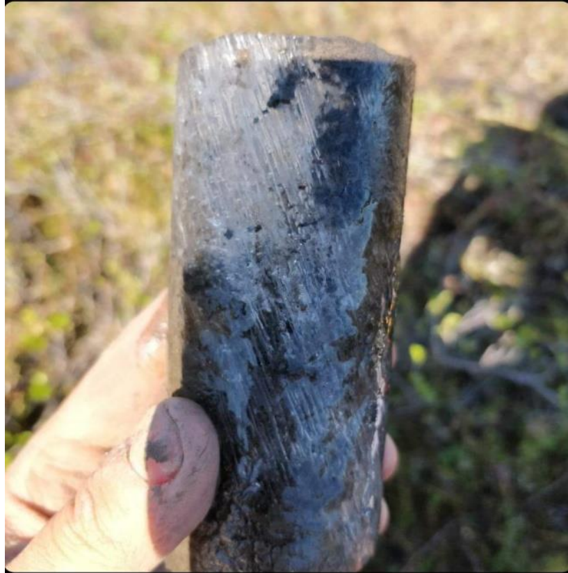
Figure 2.15: Ice-rich permafrost core taken from SSL-6 taken near the end of June of 2021.
