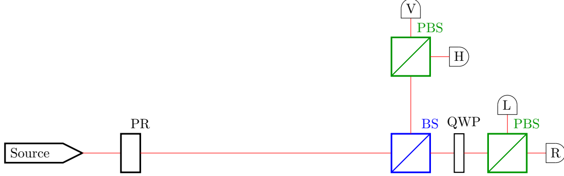
Figure 3.2: Conceptual diagram of the source and detector setup of the 3-state protocol. See the caption of Fig. 3.1 for component descriptions.
