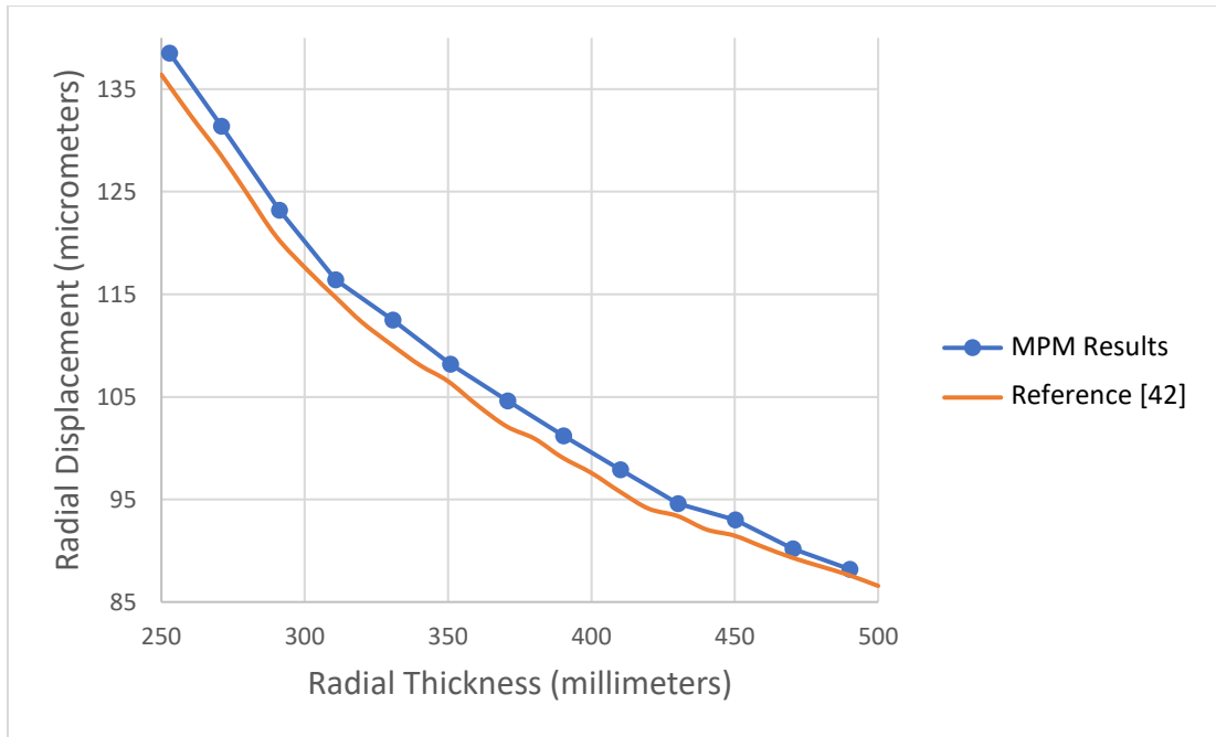
Figure 3.5 Radial displacement through the cylinders thickness. Results compared between MPM study and elastodynamic solution in study [42]
