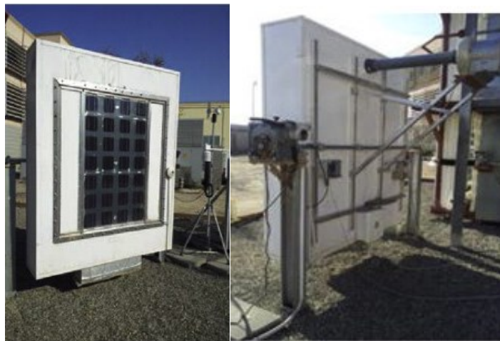
Figure 36 front and rear view of outdoor experimental setup for BIPV window TSET determination [71]
