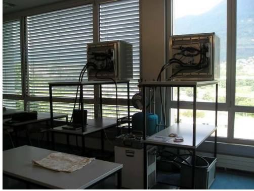
Figure 37 transportable calorimeter for in-situ measure of TSET [73]
