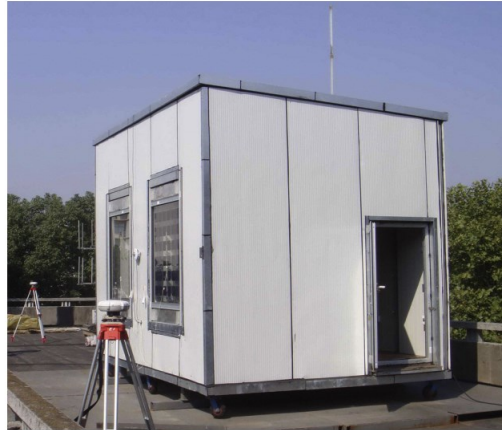
Figure 41 Experimental setup for BIPV module TSET determination [51]
