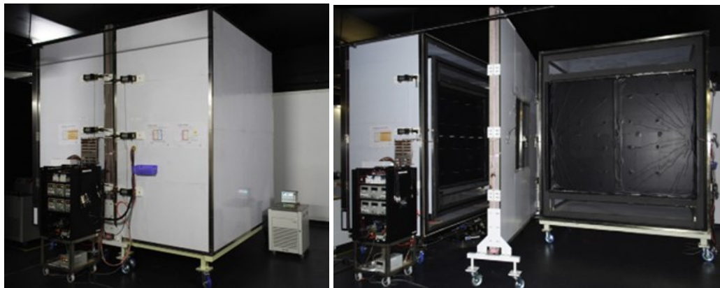
Figure 31 General view of SERIS chamber system when it is under test and the inside view from left to right respectively [60]
