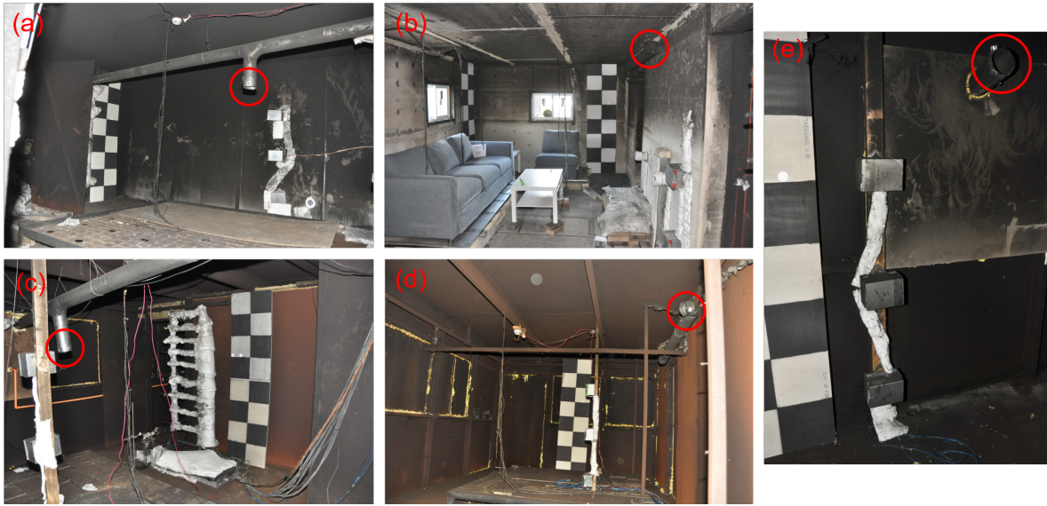
Figure 3.4: Images of ventilation ports: a) kitchen supply, b) fire room supply, c) small bedroom supply, d) large bedroom supply, and e) upper floor exhaust.
