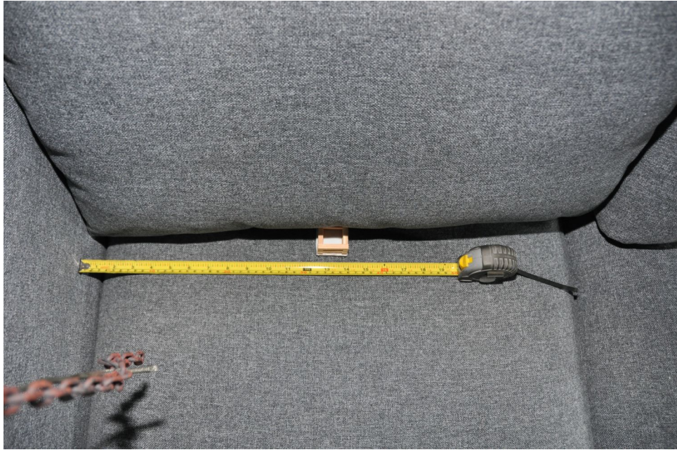
Figure 3.9: Image of the Type 4 igniter wood crib in position on the first couch cushion.
