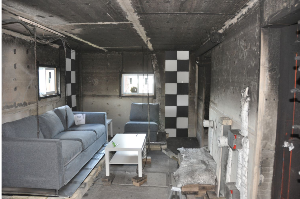
Figure 3.3: Image of the fire room setup prior to a test.
