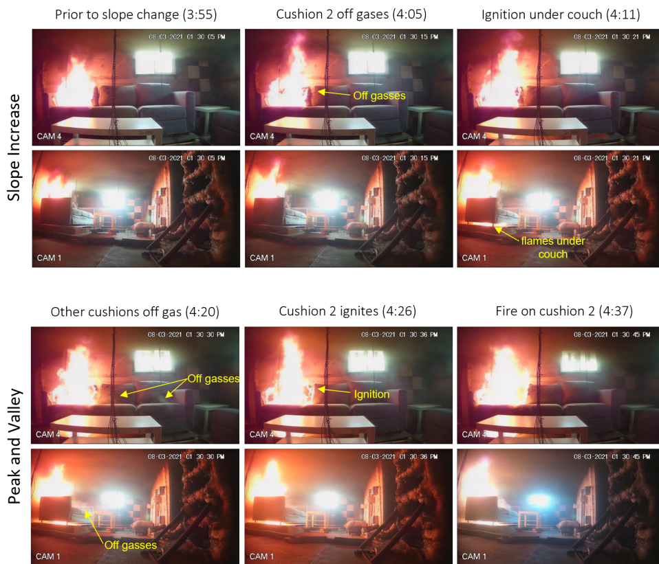
Figure 4.11: Plot of MLR from the baseline HVAC test with images of the fire during the slope increase and the local peak and valley.
