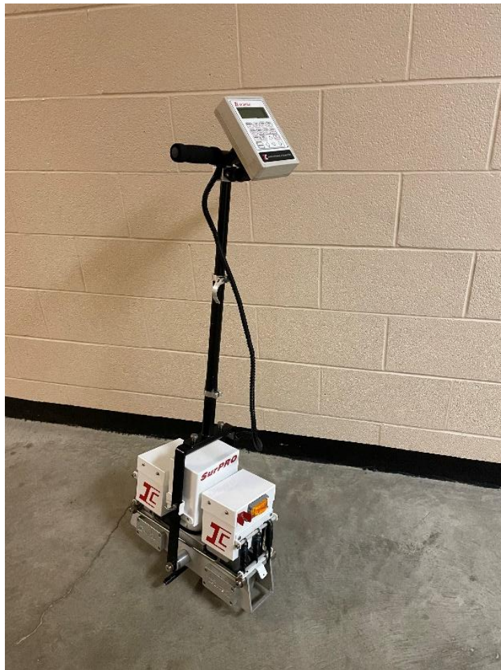
Figure 7. SurPRO 4000 Inclinometer-Based Profiler
