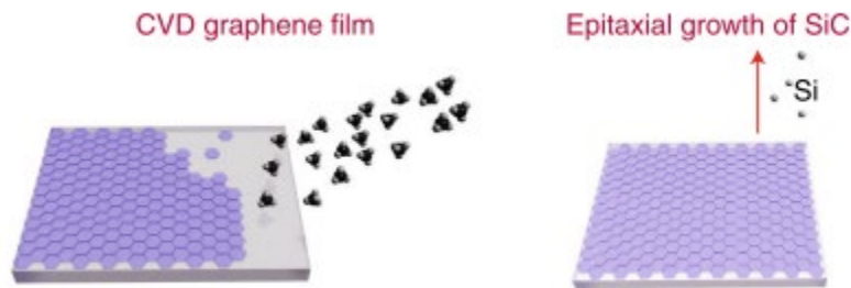
Figure 2-8. Production of graphene with CVD and Epitaxial method[82]
