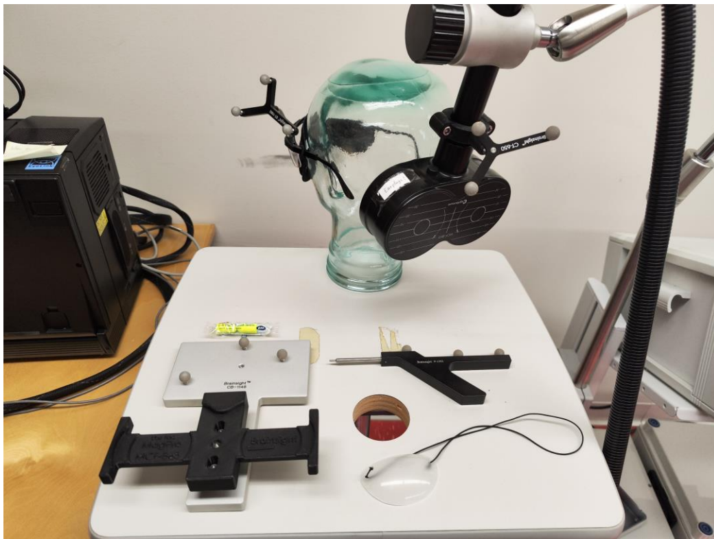
Figure 2-4. TMS apparatus, featuring a figure-of-eight coil (MCF-B65, MagVenture, Denmark). For a detailed description of TMS apparatus, please refer to the caption for Figure 6-1 in Chapter 6.
