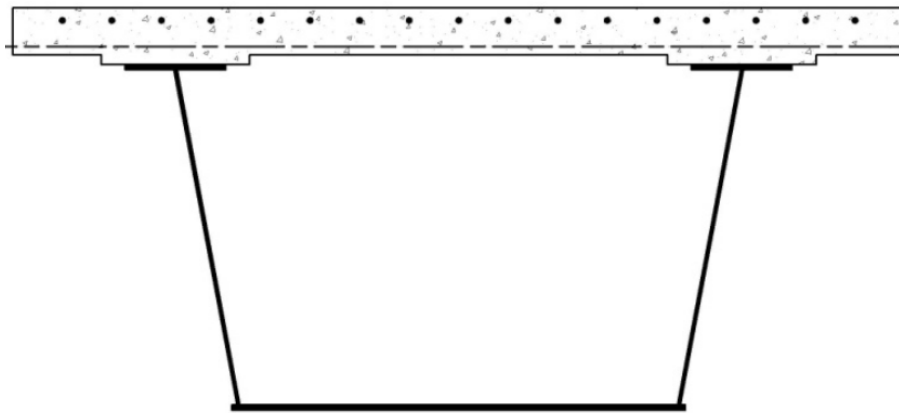
Figure 5-1. Cross section of a typical box girder
