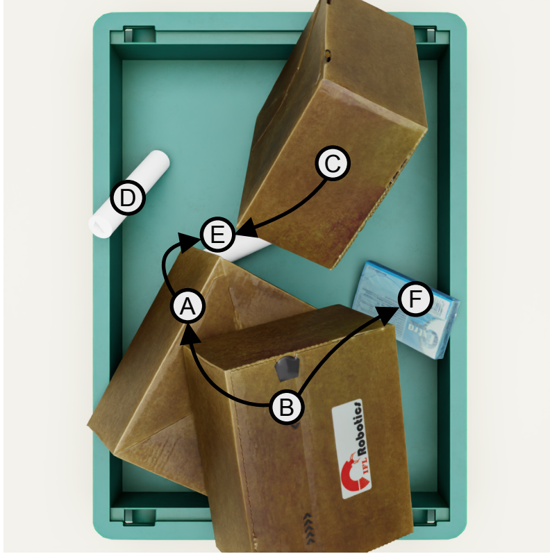
Figure 3.1: An RGB image from a simulation of a set of objects in a scene, with the relationships between objects shown with annotations illustrating G_{\rightarrow}^s . Object E is obstructed by object C and obstructed by object A, which is obstructed by object B. The image without annotation is from the MetaGraspNetV2 [4] dataset.
