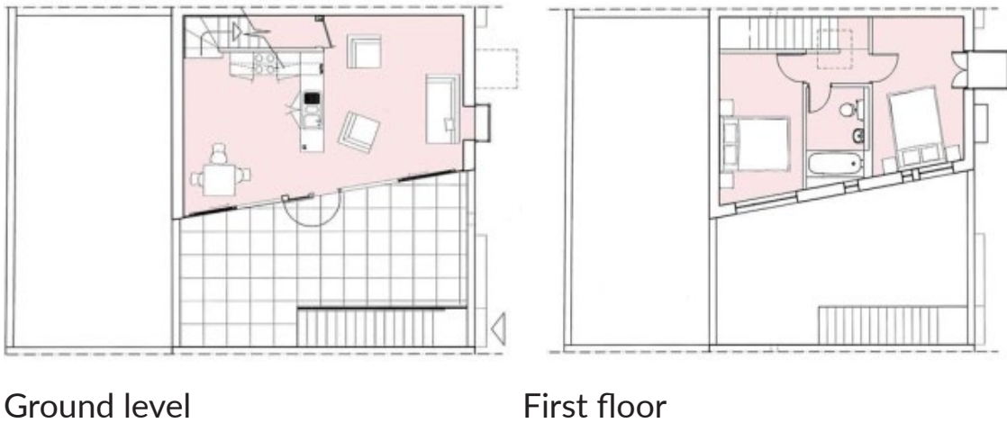
Fig 3.10 Donnybrook Quarter Floor plan of duplex units
