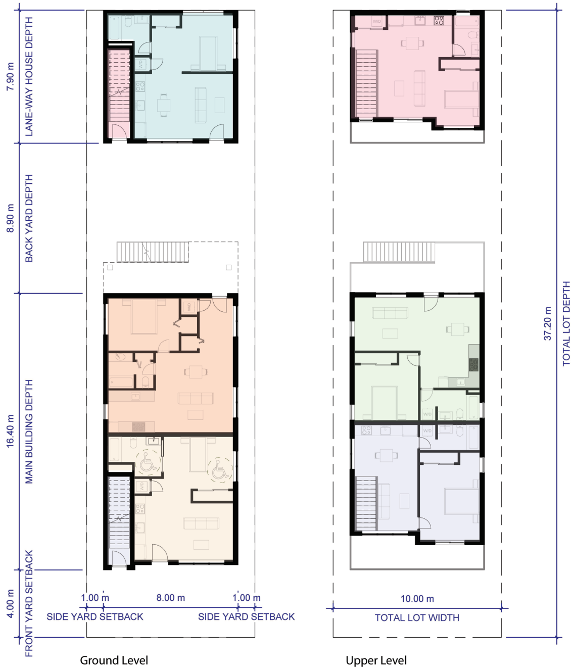
Fig 5.6 Vancouver Special 2.0 floor plans
