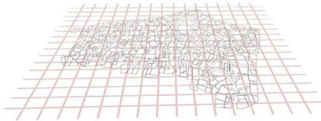
将场地用3m×3m的方格布满并几何化场地 使每家西南角朝向麦加 Cover and geometrize the site with 3m x 3m square Each house faces mecca in the southwest corner
