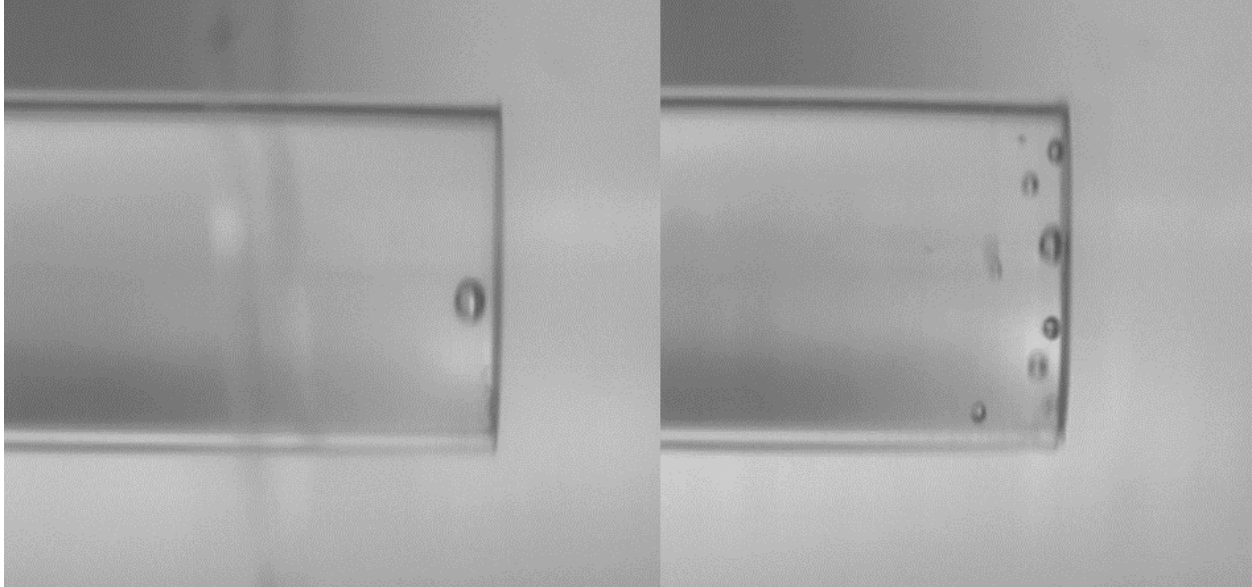
Fig 4 High-speed image of a test producing an individual cavitation bubble (left) and a test producing a cavitation bubble cluster (right)
