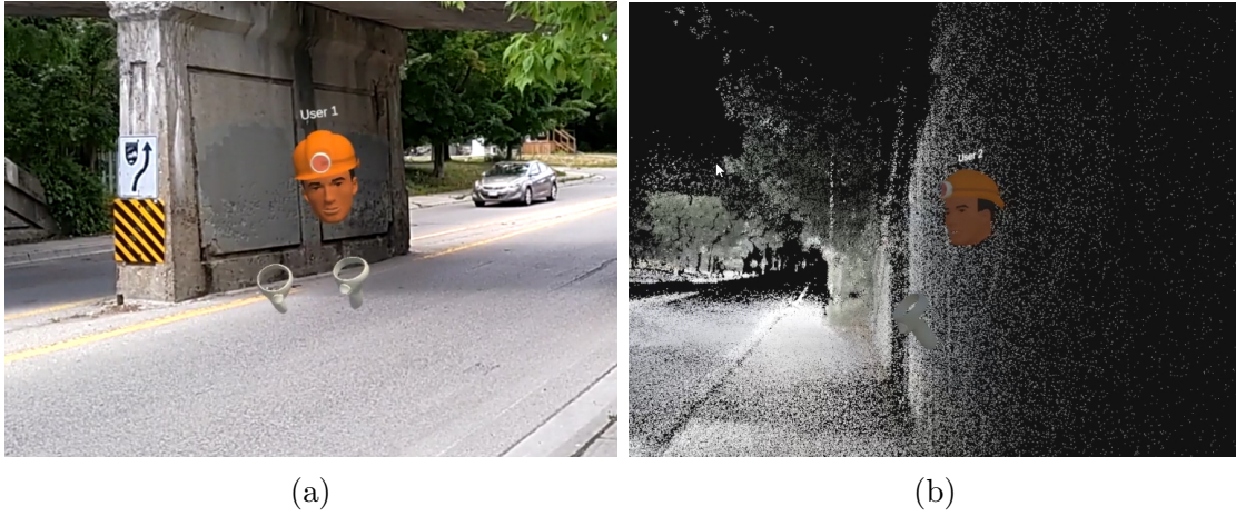
Figure 5.9: Spatially aware collaboration in MR/VR using 3D avatars: Each user perceives other users as being present in their environment through avatars, allowing them to monitor hand and head positions. Screenshots in (a) and (b) illustrate the perspective of an on-site MR user and a remote VR user, respectively.
