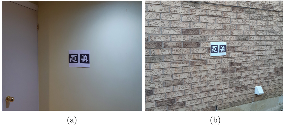
Figure 3.7: Evaluating the measurement accuracy of HL2 depending on a working distance under (a) indoor and (b) outdoor setting. Note that fiducial markers are used for automated detection.
