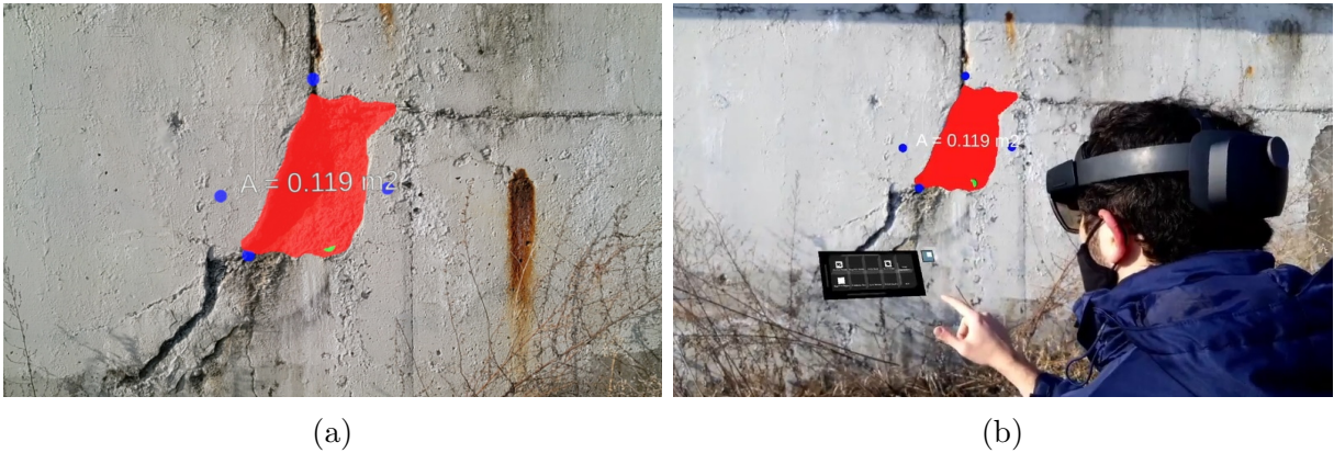
Figure 3.1: The proposed XRIV system for damage area measurement enabled through the HoloLens 2. Image (a) was captured using the HoloLens 2, while image (b) was captured using Spectator View.
