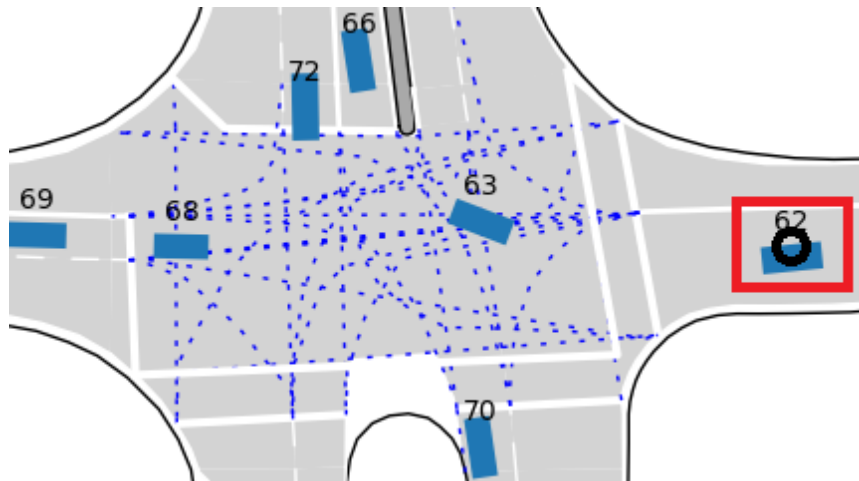
Figure 3.15: An illustration of a vehicle (red square) failing to maintain a target speed over a waypoint (black circle).
