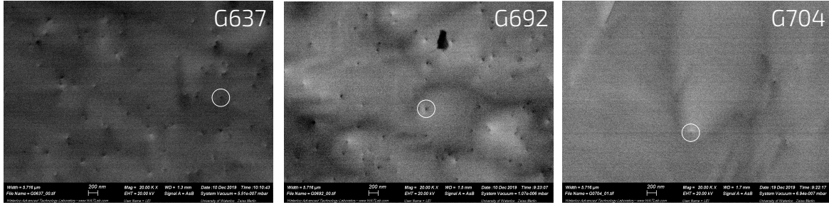
Figure 2.2: The characterization of TDD using scanning electron microscopy-electron channeling contrast imaging (SEM-ECCI) for wafers G637, G692, and G704 as indicated in the figure. White circles indicate a representative threading dislocation defect at the surface of each wafer. Details of the heterostructures are given in Table 2.3. Images and TDD characterization performed by Yinqiu Shi.
