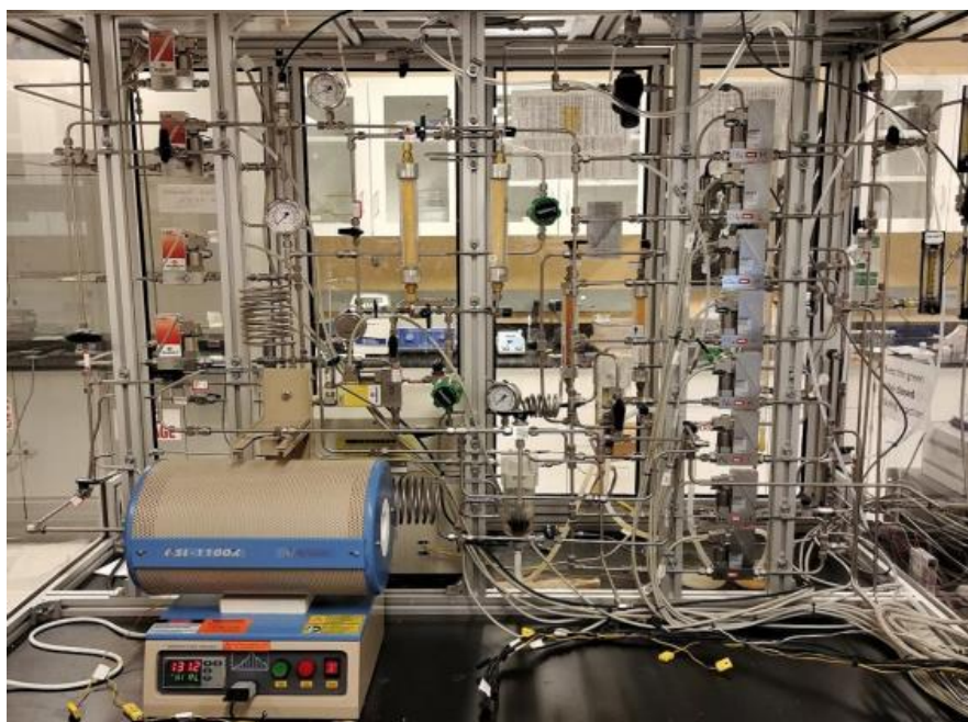
Figure 3-6 Flow system conducted for catalytic performance tests.
