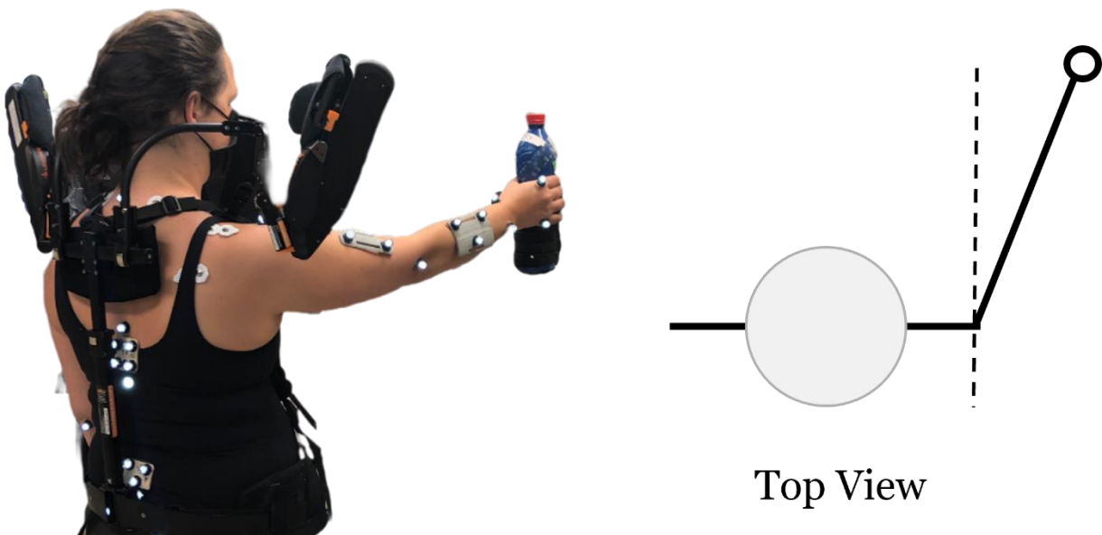
Figure 10. Representative EMG reference task (left), with a top view of the participant's arm posture (right). The top view shows the arm deviated 30 degrees clockwise from the sagittal plane.
