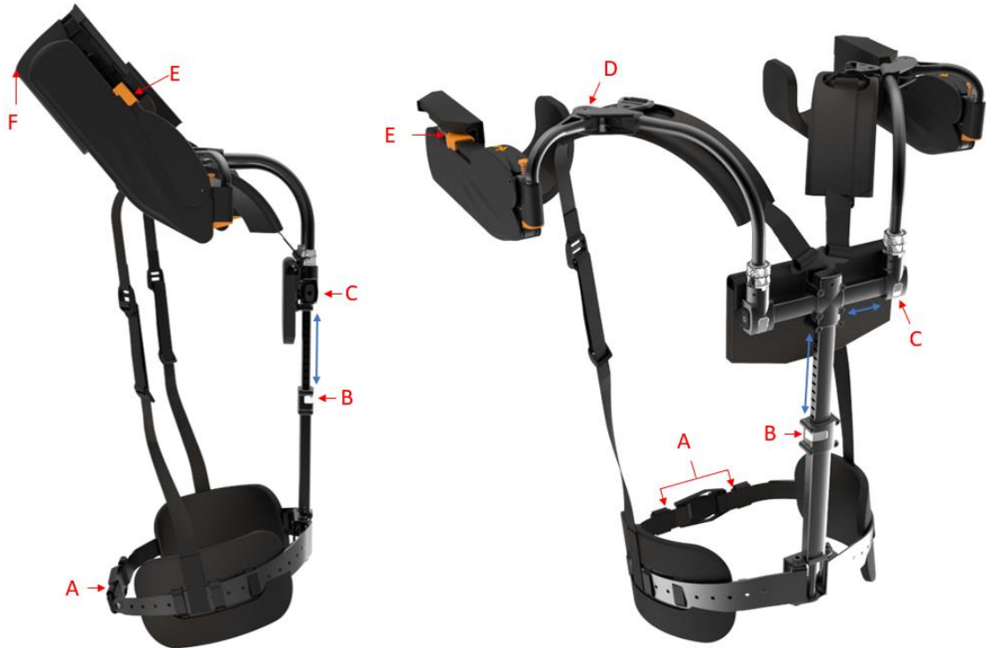
Figure 8. Levitate exoskeleton with labelled adjustable parts. (A) Waist belt, (B) superior inferior back, (C) medial lateral, (D) shoulder rotation, (E) cuff length adjustment, and (F) end of cuff. Images from: https://www.levitatetech.com/
