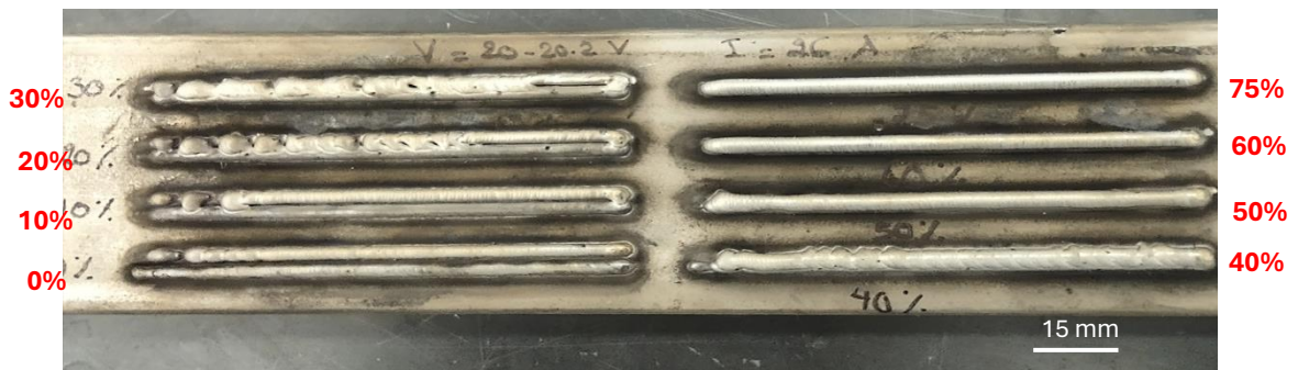
Figure 6-10: Weld beads at a current of 26 A for overlap percentages of 0, 10, 20, 30, 40, 50, 60, and 75 %
