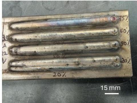
Figure 6-11: Weld beads at a current of 35 A for overlap percentages of 20, 50, 60, and 75 % (bottom to top)
