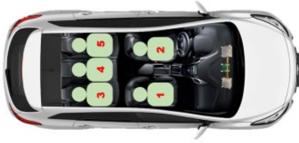
Figure D. 4: The radar setup in [70]. Seat 3 and seat 4 have the same time distance from the radar. The discrimination of these two seats is possible by having more receivers.
