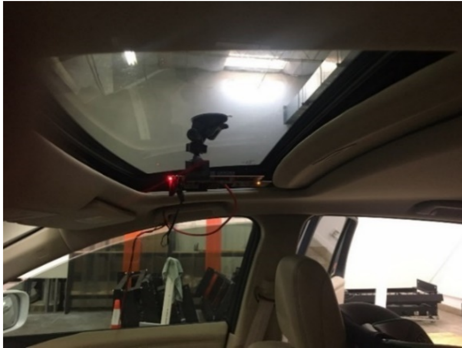
Figure 4.13: Radar setup inside the vehicle for occupancy detection.
