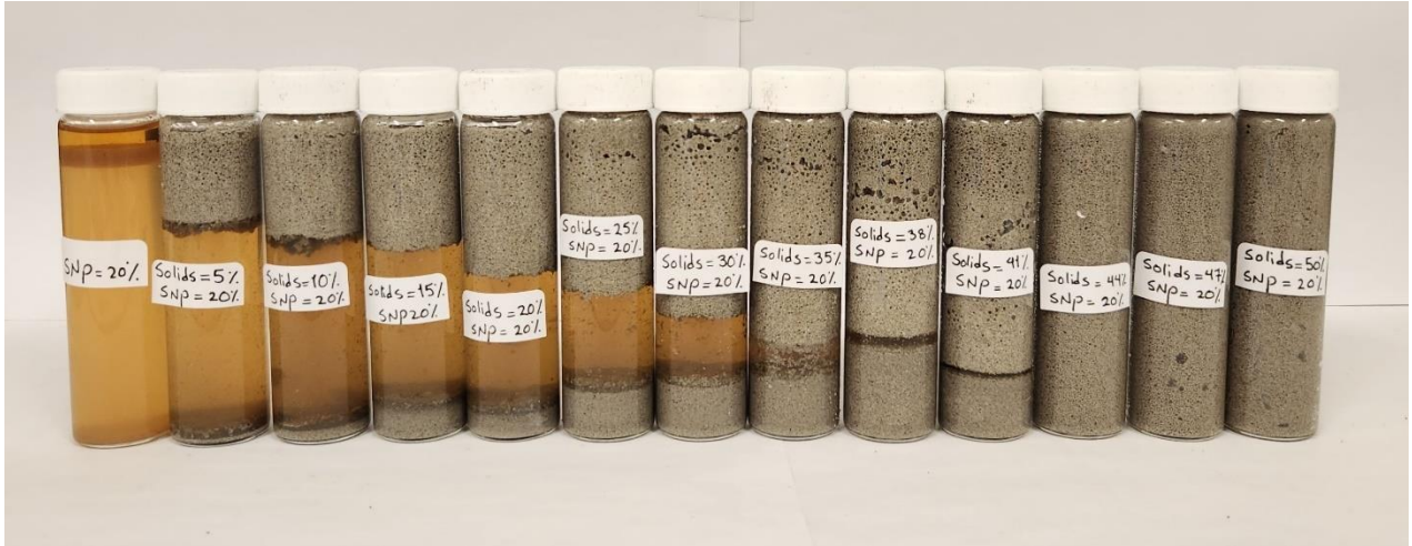
Figure 42 Samples of suspensions of SG hollow spheres in SNP dispersion, with SNP concentration of approximately 20 wt%
