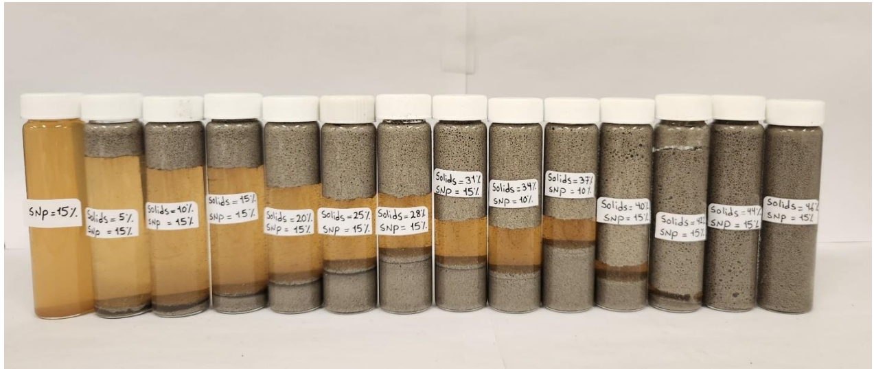
Figure 41 Samples of suspensions of SG hollow spheres in SNP dispersion, with SNP concentration of approximately 15 wt%
