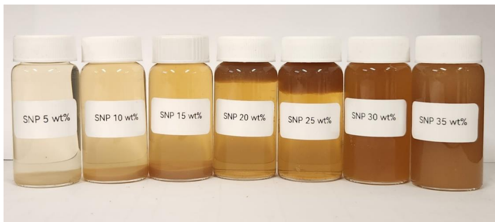
Figure 11 Samples of SNP dispersions in the order of increasing SNP concentration from approximately 5 to 35 wt%.
