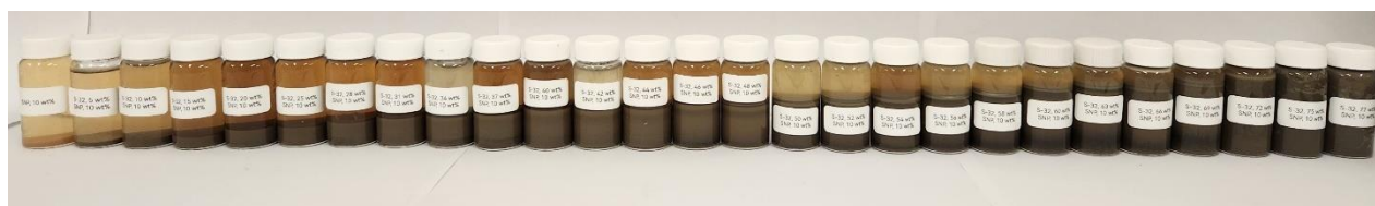
Figure 47 Samples of suspensions of S-32 solo spheres in SNP dispersion, with SNP concentration of 10 wt%
