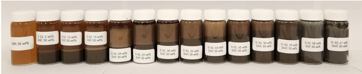
Figure 51 Samples of suspensions of S-32 solo spheres in SNP dispersion, with SNP concentration of 30 wt%
