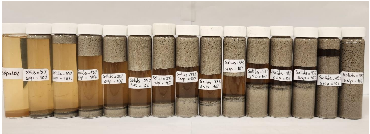
Figure 40 Samples of suspensions of SG hollow spheres in SNP dispersion, with SNP concentration of approximately 10 wt%
