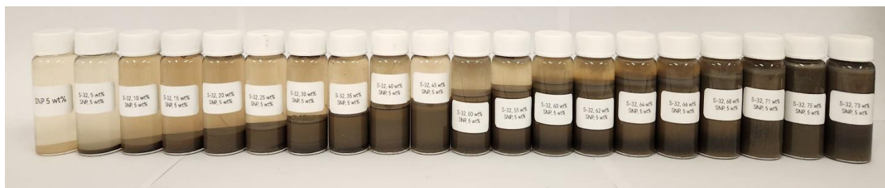
Figure 46 Samples of suspensions of S-32 solo spheres in SNP dispersion, with SNP concentration of 5 wt%
