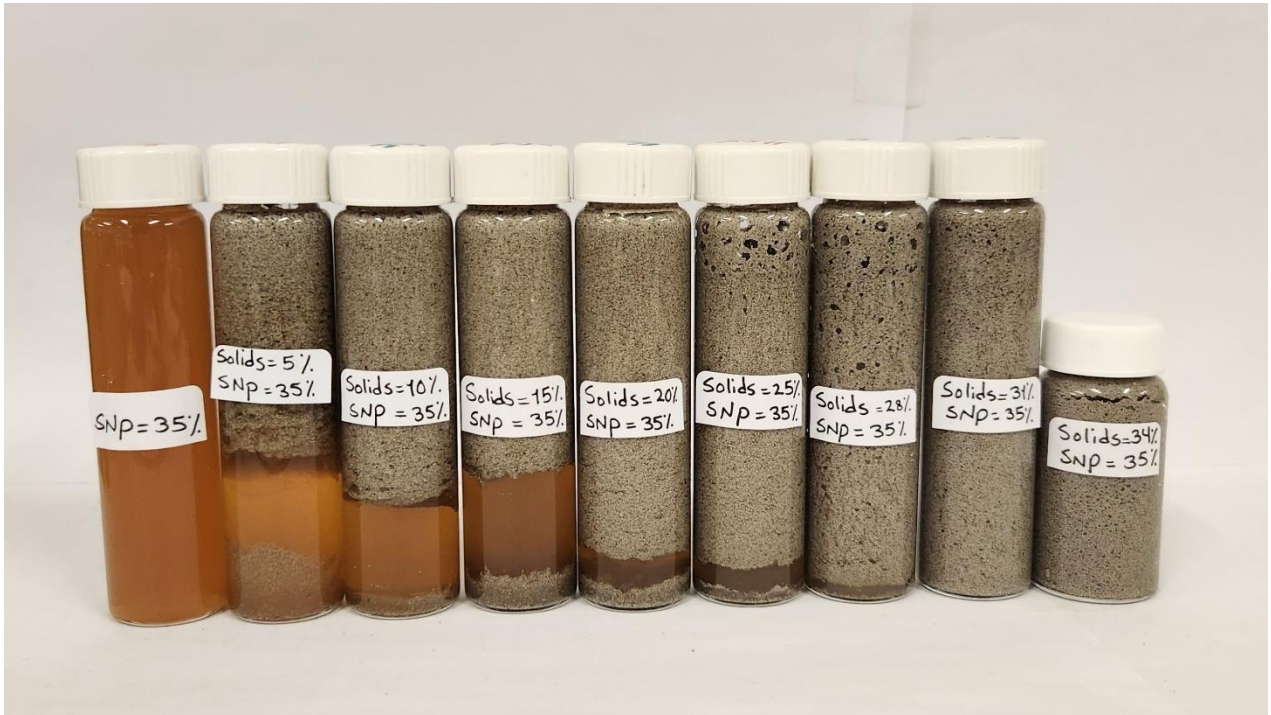
Figure 45 Samples of suspensions of SG hollow spheres in SNP dispersion, with SNP concentration of approximately 35 wt%
