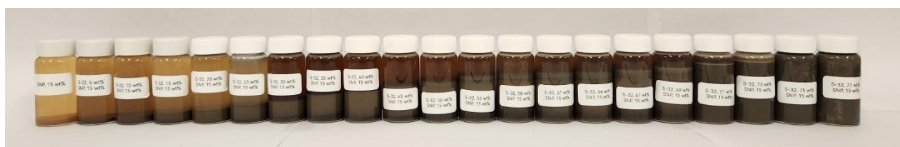
Figure 48 Samples of suspensions of S-32 solo spheres in SNP dispersion, with SNP concentration of 15 wt%
