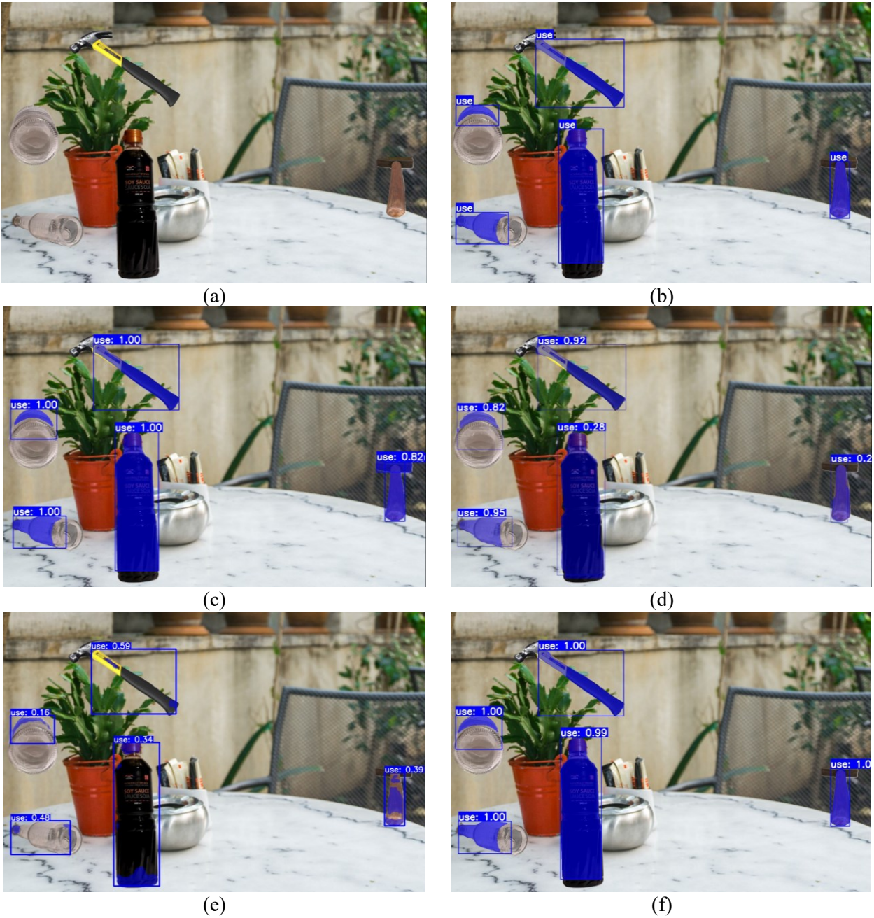
Figure 4.8: Instance segmentation predictions for the task-region detection category, for the use class: (a) original input image, and (b) ground truth or target. (c) to (f) are the predictions from Mask R-CNN, YOLACT, YOLOv5s-Seg, and MAD-Net, respectively.
