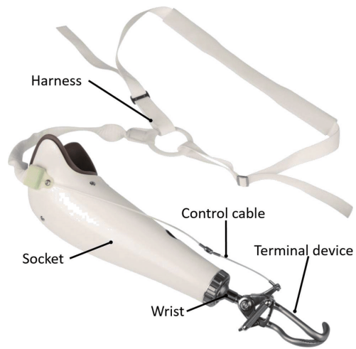
Figure 1.2: Parts of a single-control system, body-powered cable-operated prosthesis with a hook terminal device. The terminal device is controlled through a control cable, that is connected to the shoulder harness. Adapted from [24].
