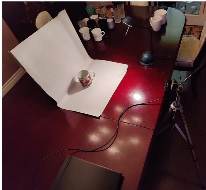
Figure 3.5: Camera setup to capture real single-object RGB images with the OAK-D Camera.
