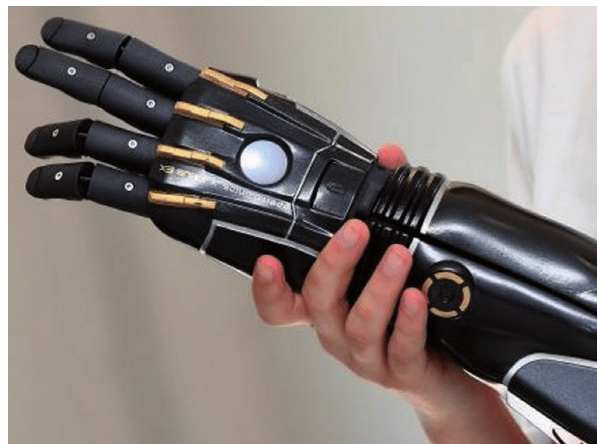
Figure 1.5: Example of a myoelectric prosthesis: Open Bionics' Hero Arm. The circular button on the back of the terminal device is the program switch to cycle through an alternative set of grasp types. Adapted from [24].
