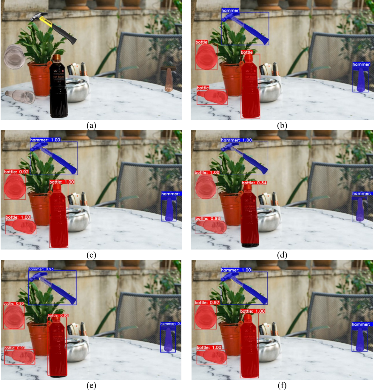
Figure 4.4: Instance segmentation predictions for the object (bottles, cups, etc.) detection category: (a) original input image, and (b) ground truth or target. (c) to (f) are predictions from Mask R-CNN, YOLACT, YOLOv5s-Seg, and MAD-Net, respectively.
