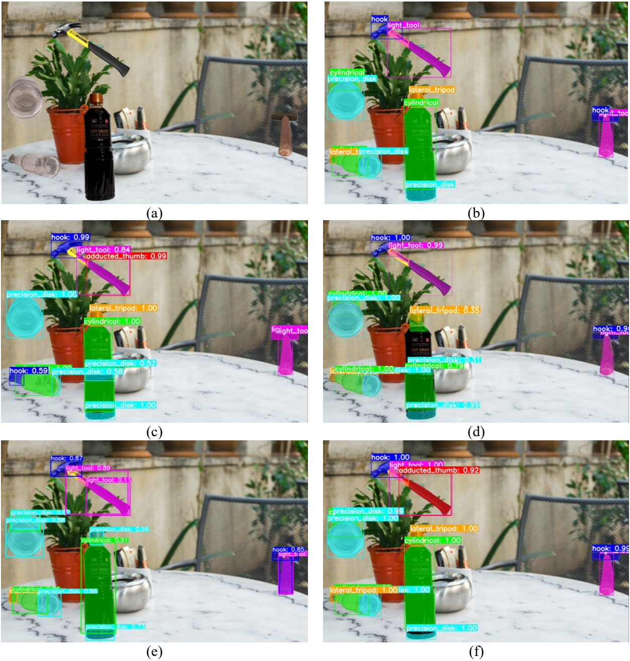
Figure 4.5: Instance segmentation predictions for the grasp-type detection category: (a) original input image, and (b) ground truth or target. (c) to (f) are predictions from Mask R-CNN, YOLACT, YOLOv5s-Seg, and MAD-Net, respectively.
