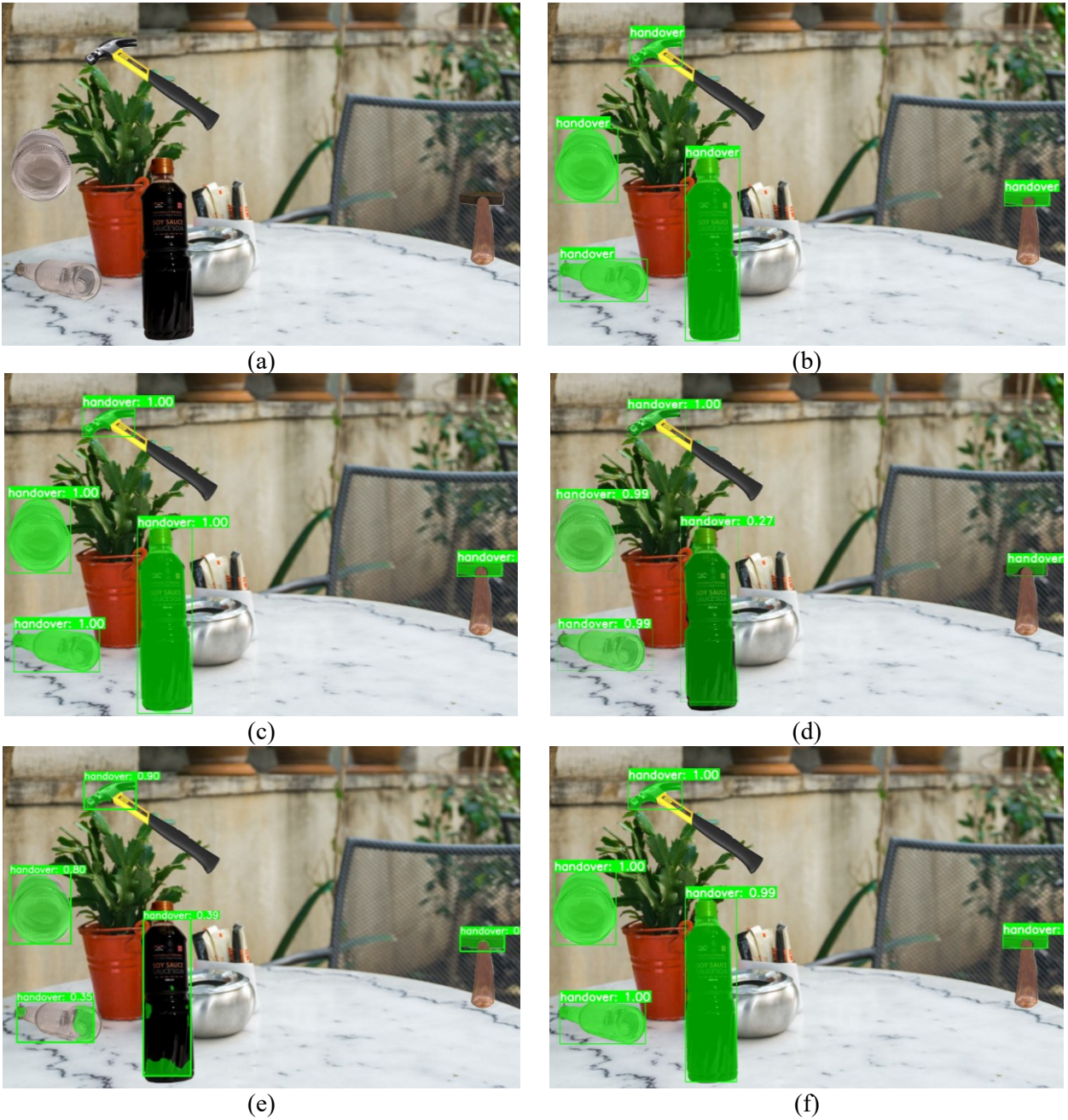
Figure 4.7: Instance segmentation predictions for the task-region detection category, for the handover class: (a) original input image, and (b) ground truth or target. (c) to (f) are predictions from Mask R-CNN, YOLACT, YOLOv5s-Seg, and MAD-Net, respectively.
