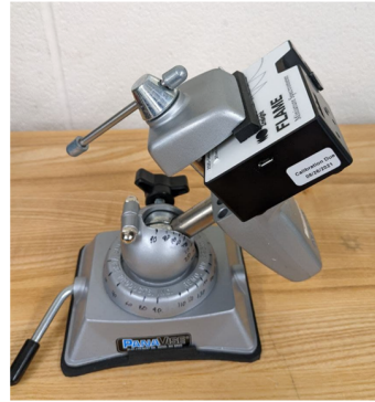
Figure 2.22: a) Light pollution measurement device for the dark detection method. A multimode fiber, a bandpass filter ( 790 \pm 5\text{nm} ), a rotating clamp and a SPAD detector are used to measure the background counts. b) Light pollution measurement device for the spectroscopy method. A mini spectrometer and a rotating clamp are used to take the spectra of light coming from the parking lot area. Both photos are taken by my colleague, Paul Godin.
