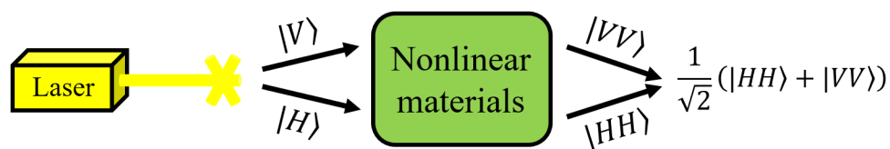
Figure 3.1: A schematic diagram showing the process of generating entangled states. We utilize nonlinear materials that can perform SPDC. The entanglement of photon pairs is achieved by building an interferometer.
