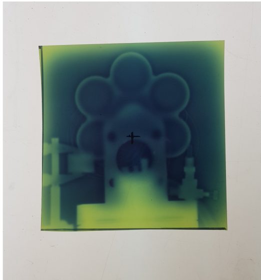
Figure 4.9: A proton-radiated photograph of the radiation test setup. The film was also exposed to the proton radiation by being positioned in front of the test setup, along the proton beam path.
