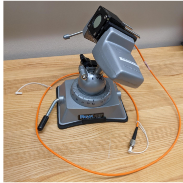
Figure 2.22: a) Light pollution measurement device for the dark detection method. A multimode fiber, a bandpass filter ( 790 \pm 5\text{nm} ), a rotating clamp and a SPAD detector are used to measure the background counts. b) Light pollution measurement device for the spectroscopy method. A mini spectrometer and a rotating clamp are used to take the spectra of light coming from the parking lot area. Both photos are taken by my colleague, Paul Godin.
