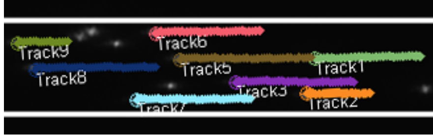
Figure 4.3 Example of particle tracking measurements in microchannel flow.
