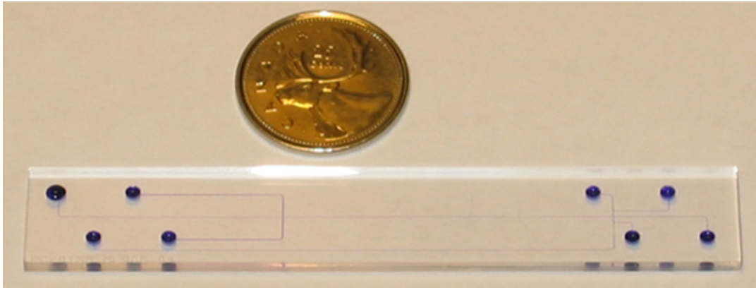
Figure 5.1 Micralyne microfluidic chip filled with dark ink to enhance the channels.
