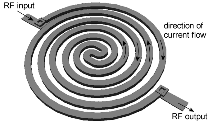
Fig. 6.1: Schematic indicating the direction of current flow for a single metal layer MEMS inductor.
