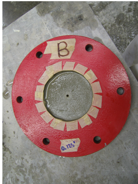
Figure 4-5: Lined post test bottom plate where blow-out has occurred.
