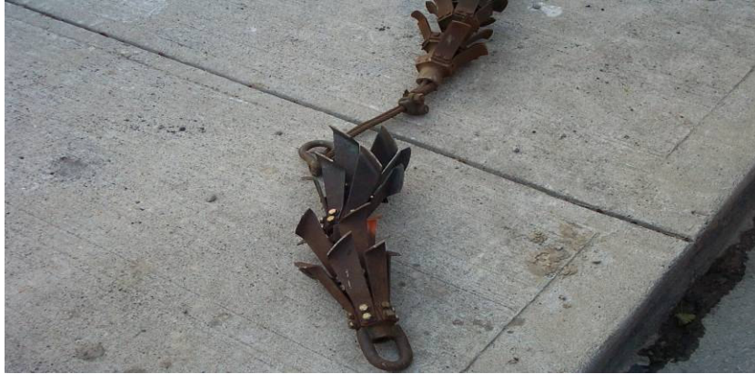
Figure 2-3: Mechanical scraping tool used to clean internal corrosion products.
