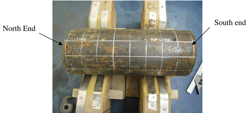
Figure 4-10: Pipe section #1 showing grid pattern for corrosion potential measurements.
