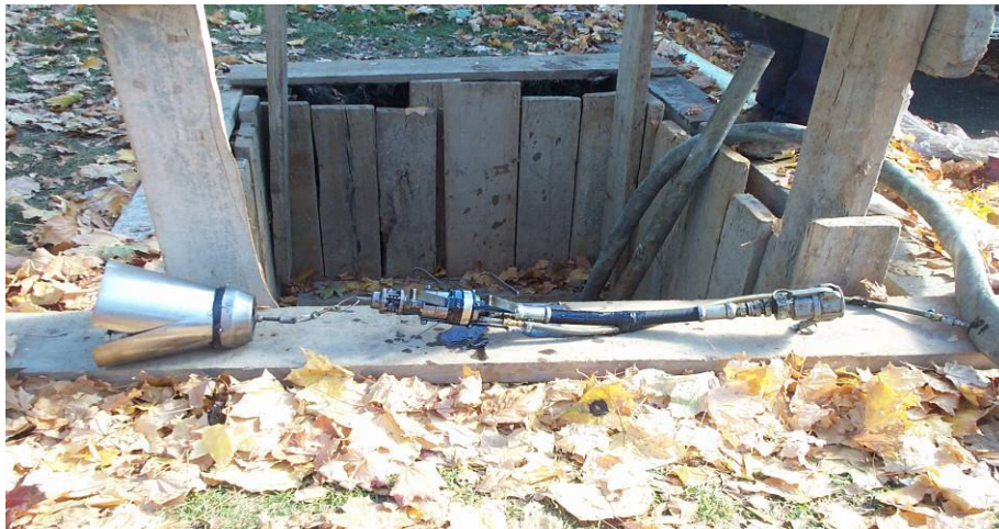
Figure 2-5: Mechanical trowelling device used to apply mortar to the inside of watermains.
