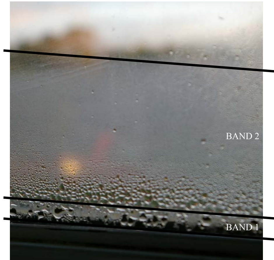
Figure 3.1: Multiple bands of condensation with run-off
