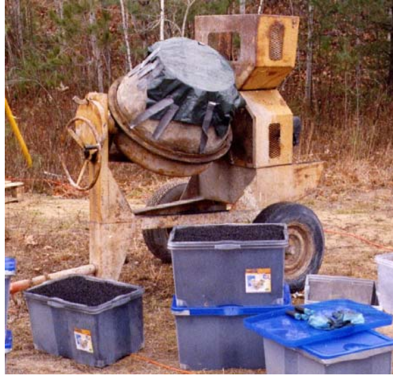
Figure 2.17. Photograph of cement mixer used to homogenize activated carbon and high density polyethylene containers filled with activated carbon.
