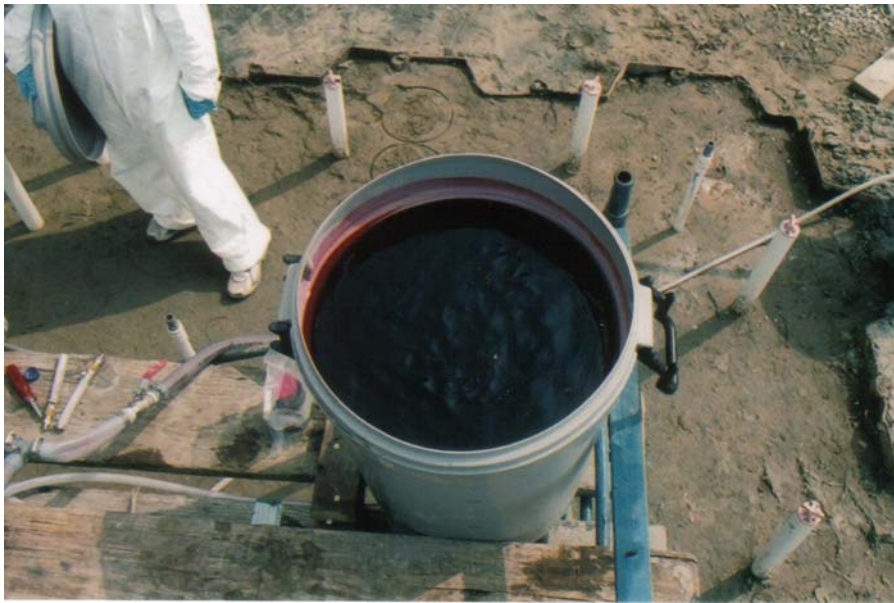
Figure 2.13. Photograph of the dyed contaminant mixture in high density polyethylene container prior to injection.
