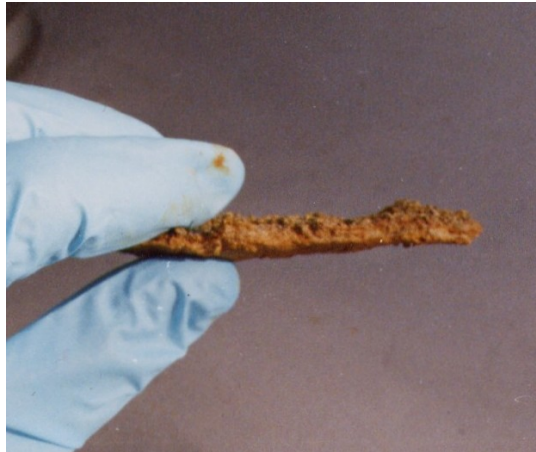
Figure 3.14. Photograph showing colour and thickness of precipitate formed in water filter.
