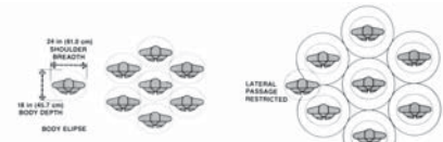
Figure 2-4 (left) Illustration of Fruin's "touch zone" based on a "body ellipse" buffer zone with a minor axis related to body depth and a major axis related to shoulder breadth, allowing a spacing area of 3 sq ft, or 0.29 sq m, per person. Below this boundary the frequency of body contact between pedestrians is increased. Figures 2-4 to 2-7 adapted from Fruin, Pedestrian Planning and Design , 1971. Figure 2-5 (right) Illustration of Fruin's "no touch zone," based on an expanded intersperser spacing of 36 in, or 91.4 cm, and a 7 sq ft, or 0.65 sq m, area per person. Fruin contends that body contact can be avoided between 3 and 7 sq ft, or 0.29 to 0.65 sq m, per person.
