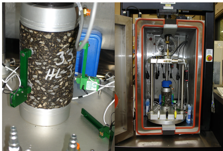
Figure 5.17 Dynamic Modulus Testing Setup in the Interlaken.
