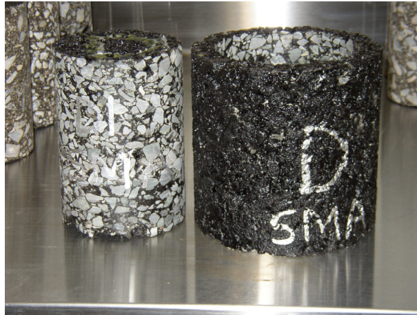
Figure 5.20 Core of the SMA G mix and the ring remaining after the coring.
