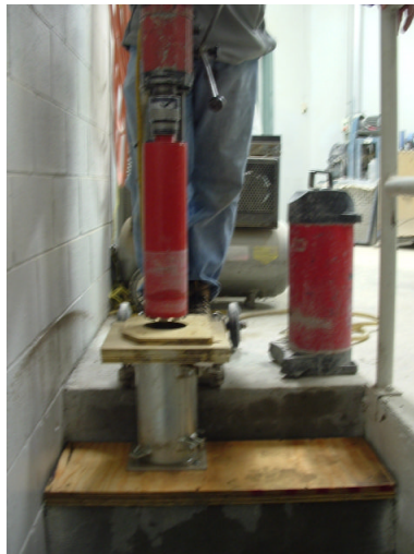
Figure 5.18 Coring System Used to Obtain 100 mm Cores from 150 mm Diameters SGC Cylinders.
