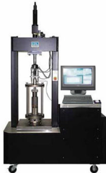
Figure 5.24 Interlaken Triaxial Test Configuration [ITC 2004] (temperature chamber is not shown).
