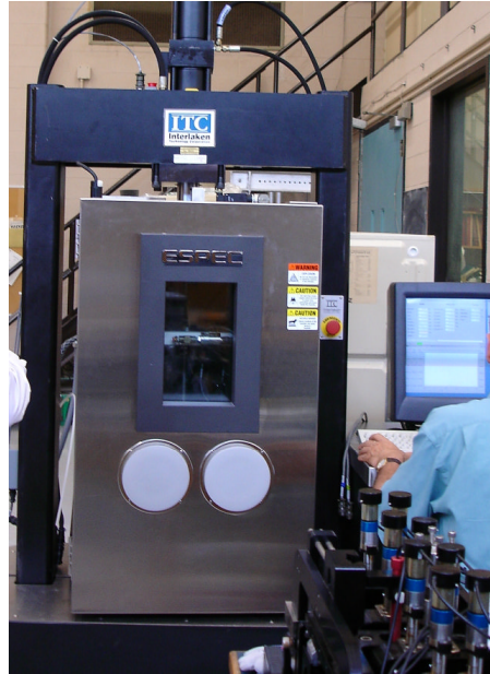
Figure 5.16 General View of the Interlaken Universal Test Machine/Simple Performance Tester.
