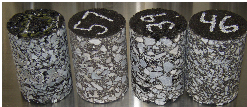
Figure 5.19 Cored Specimens of the SMA G (#D1), SP 19 D (#57), SP 19 E (# 39) and HL 3 (#46) Mixes.
