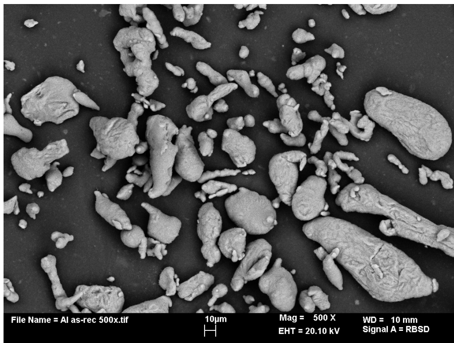
Fig. D.2 BSE micrograph of the elemental Al powder.
