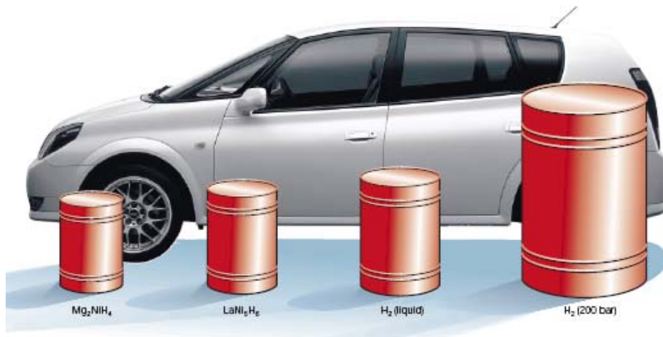
Fig. 3.1 Volume of 4kg of hydrogen compacted in different ways, with size relative to the size of a car [13].
