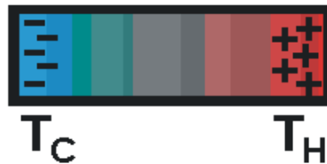
Figure 1.3 Temperature gradient between the two ends of the bar shaped thermoelectric material causes charge accumulation and potential difference between the hot end and the cold end.
