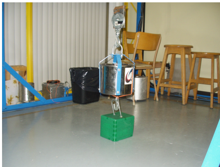
Figure 6.21: The Overhead Crane Picks Up the Object from the Workspace.
