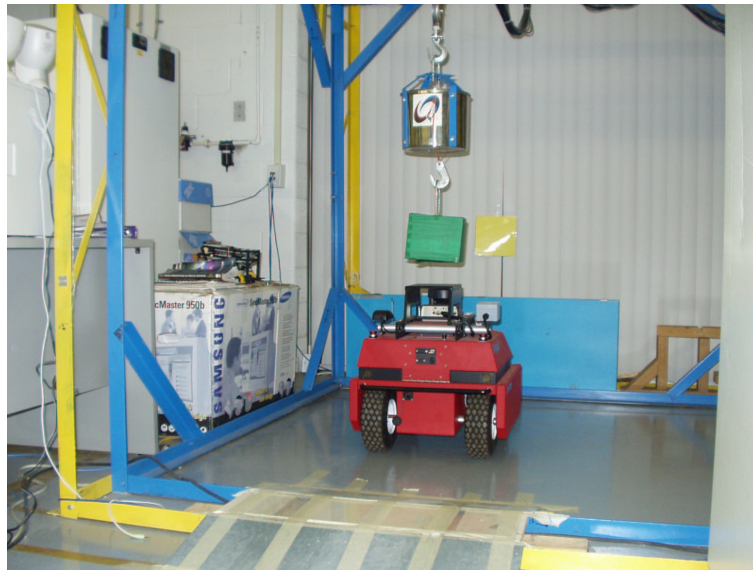
Figure 6.19: The Overhead Crane Drops the Object on Top of the Mobile Robot.
