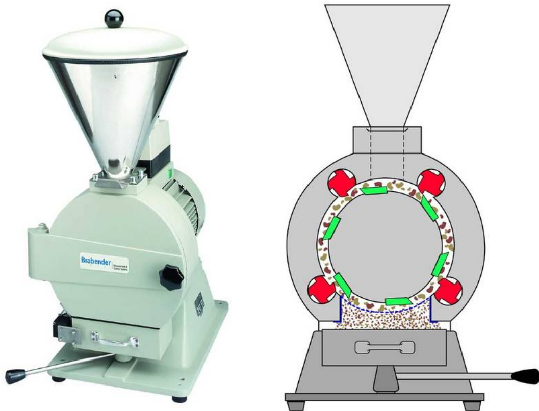
Figure 3.3: Wiley mill with six revolving and four stationary blades
