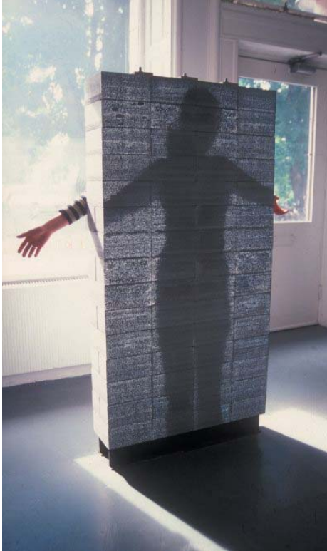
fig 3.20 Translucent concrete allows the transmission of daylight into interior spaces.
