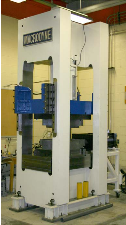
Figure 9: Macrodyne 1000-tonne hydroforming press (note that the picture does not show the s-rail die in the press)
