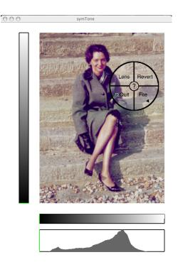
Figure 6.1: Comparison lens and file-related functions can be accessed via a pop-up transparent menu.
