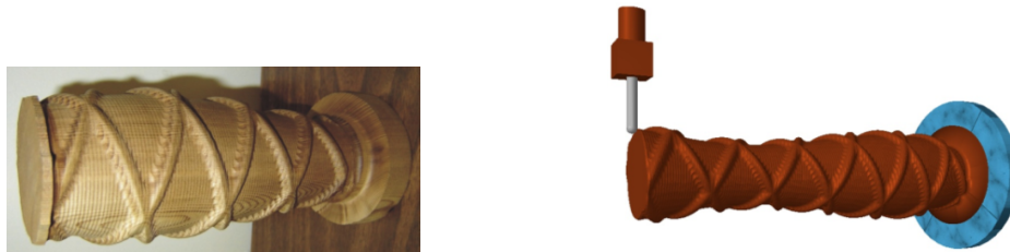
Figure 5.2: The real and virtual surface machined for [GPI + 05].
