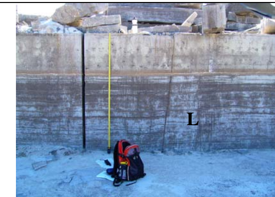
Figure 6.12F: Example of the Eramosa Member 'Marble Beds' from the OSLW Quarry. Note the decreased porosity and planar laminations (L).
