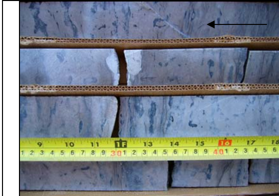
Figure 6.12A: Example of the Lions Head Member from borehole OGS-82-4. Note the low porosity. Arrow is located at the base of the core.
