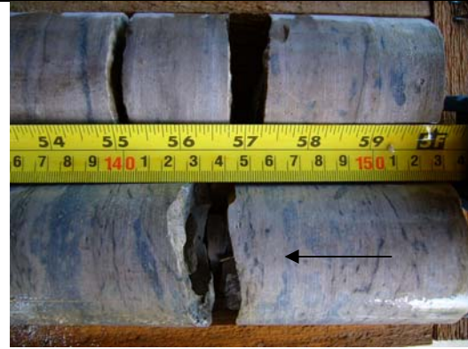
Figure 6.12D: Example of the Lions Head Member from borehole OGS-90-4. Note the low porosity. Arrow is located at the base of the core.
