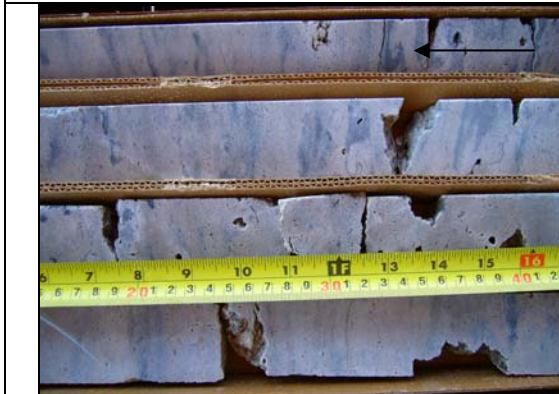
Figure 6.12B: Example of the Colpo Bay Member from borehole OGS-82-4. Note the increased vuggy porosity. Arrow is located at the base of the core.
