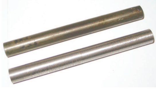
Figure 1-1: Terfenol-D rod (top) and cold-rolled steel rod (bottom).
