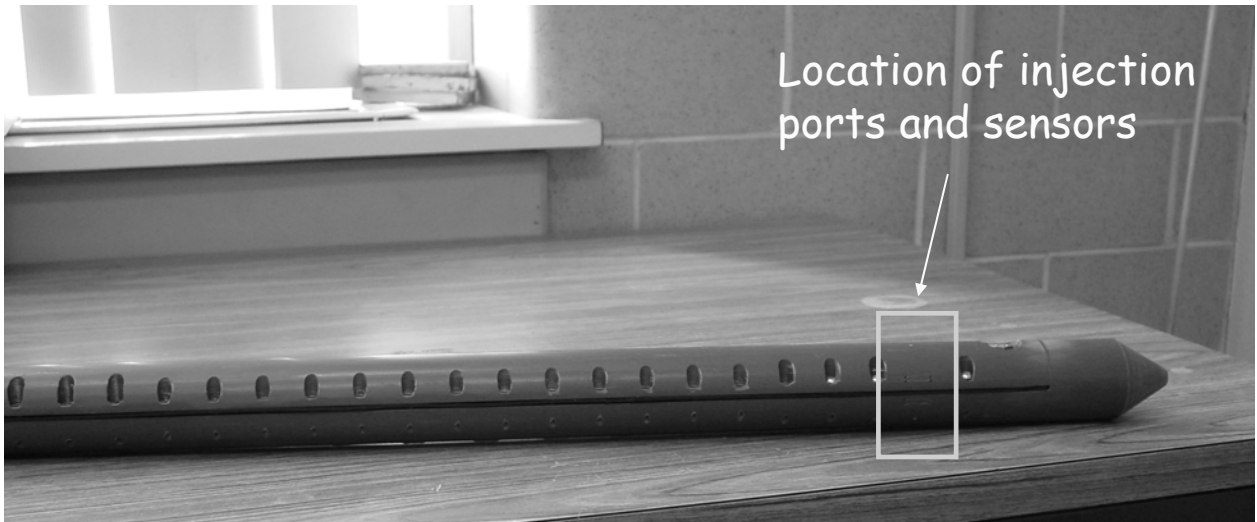
Figure 3.1 Overview picture of the redesigned PVP with location of sensors and injection ports indicated.
