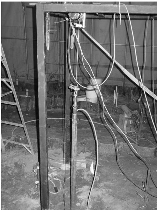
Figure 3.7 Close up of injection port and electrical conductivity sensors.
