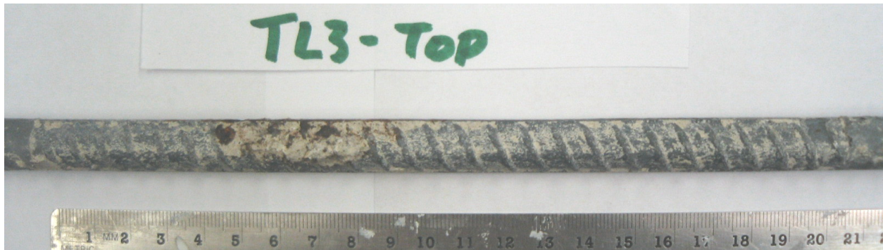
Figure 4.26: A corroded rebar removed from the TL3 concrete specimen before pickling
