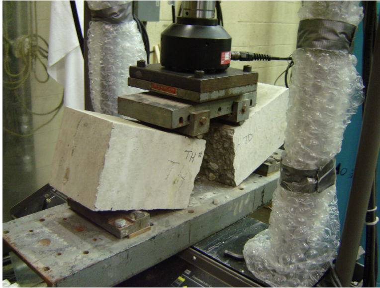
Figure 3.8: Flexural test on standard prism mode of failure
