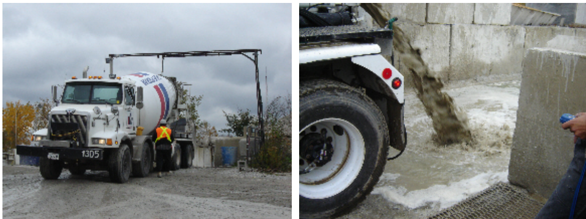
Figure 2.17: Concrete truck cleaning and rinsing at Dufferin Ready-Mix Concrete
