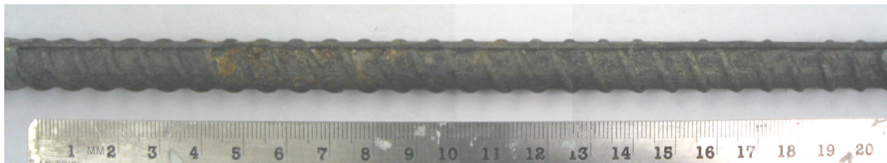
Figure 4.27: A corroded rebar removed from the TL3 concrete specimen after pickling
