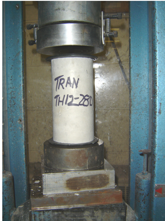
Figure 3.6: Concrete cylinder compression test
