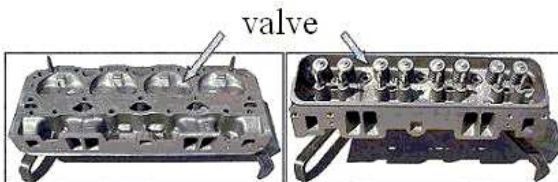
Figure 1.2: Cylinder head of an eight-valve engine as viewed from the top (right) and the bottom (left).
