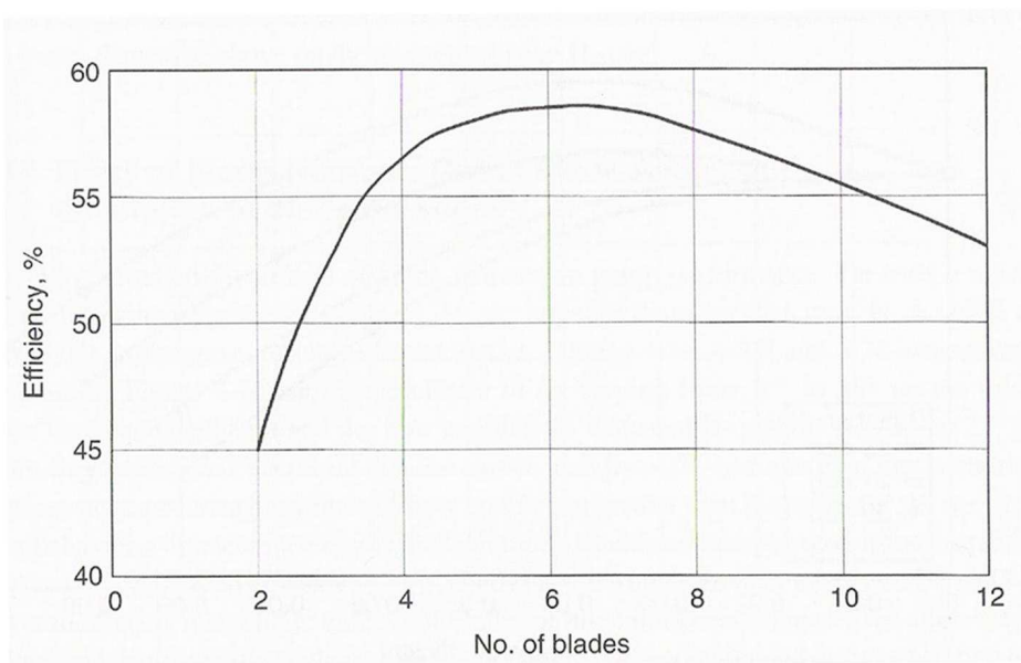
Figure 1.7: Effect of blade number on pump performance [3]
