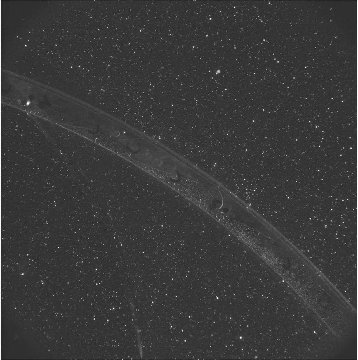
Figure 3.3: Typical PIV image of seeded flow
