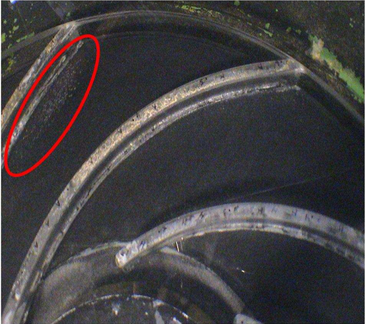
Figure 4.57: Bubbles formed and accumulated at the hub internal surface close to the suction side at 25 % of the design flow rate
