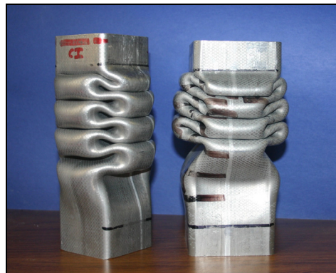
Figure 1.2: Axial crush members after impact [2].
