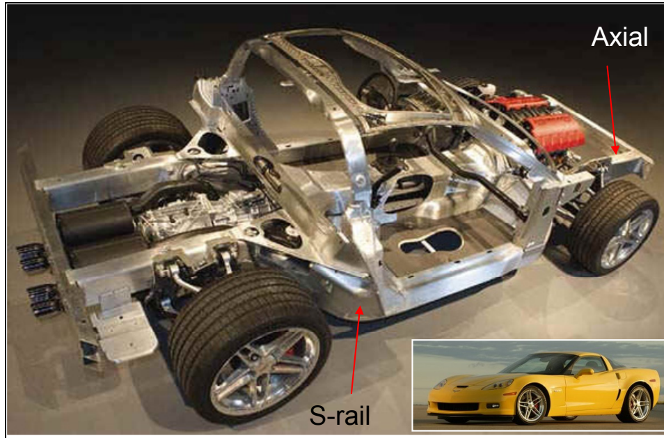
Figure 1.1: 2006 Corvette frame showing the location of a one piece aluminium hydroformed s-rail that incorporates a frontal axial crush zone [1].
