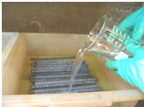
a) Adding HCl solution to steel bars
