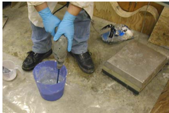
b) Epoxy mixing
