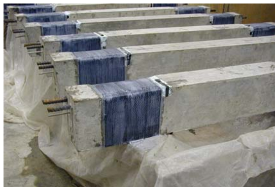
d) CFRP system curing
