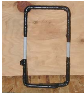
Figure 2.4: Epoxy coated stirrup covered with electrical tape at the corners
