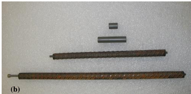
Figure 3. 2. (a) one tapped steel segment with a threaded rod, (b) two segments with two PVC pieces for isolation.
