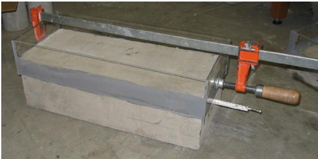
Figure 3. 5. Ponding well attachment to a concrete specimen with 50 mm cover depth.
