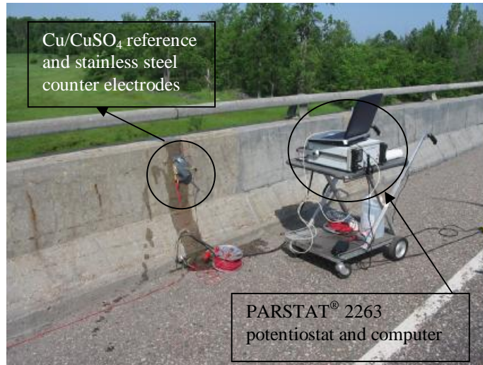
Figure 3. 28. The setup consisted of PARSTAT® 2263 potentiostat, reference and counter electrodes and the computer, used for performing electrochemical tests of the steel bars in the barrier walls, Renfrew, Ontario.
