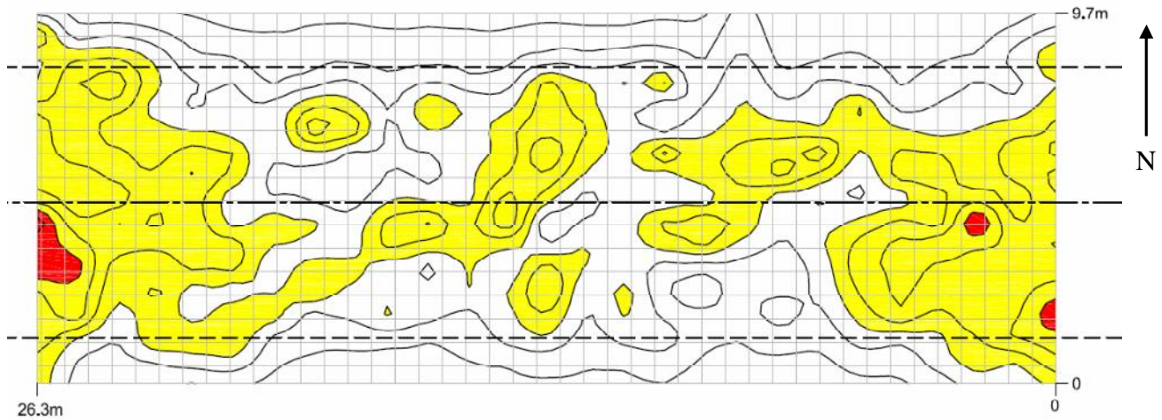
Figure 2. 7. Half-cell potential contour map, measured by CSE; Lower Elk Creek Bridge #2531, British Columbia [60].
