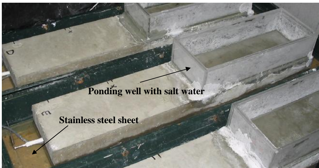
Figure 3. 3. Concrete beams in a container filled with water. A stainless steel sheet is kept at the bottom of the container as counter electrode.
