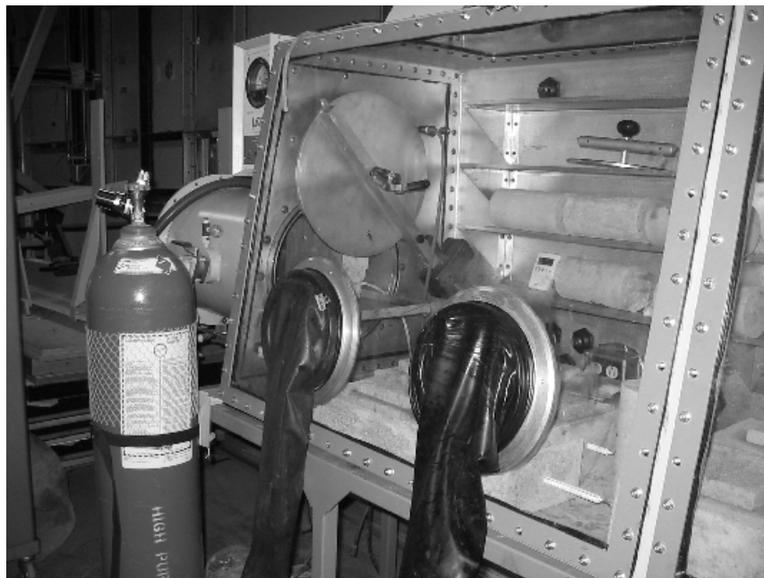
Figure 3. 8. View of the glove box used in this project to carbonate the concrete specimens.
